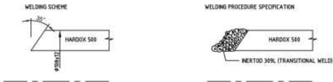
Fig. 2 Weld scheme of transitional weld
