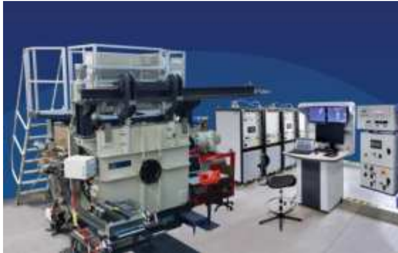
Fig.. 10 Experimental electron beam workstation for research into welding of CrMo steels
