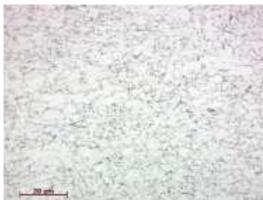
Fig. 10. Microstructure of base material S500MC
