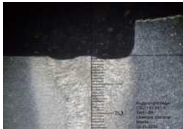
Fig. 4. Macrostructure of the weld metal
