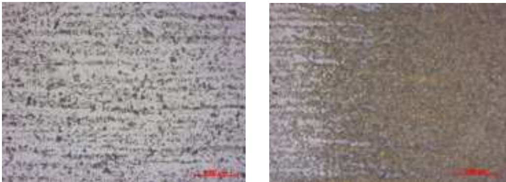
Fig. 5. Microstructure of steel 16MnCr5 – base material (left) and HAZ1 (right)
