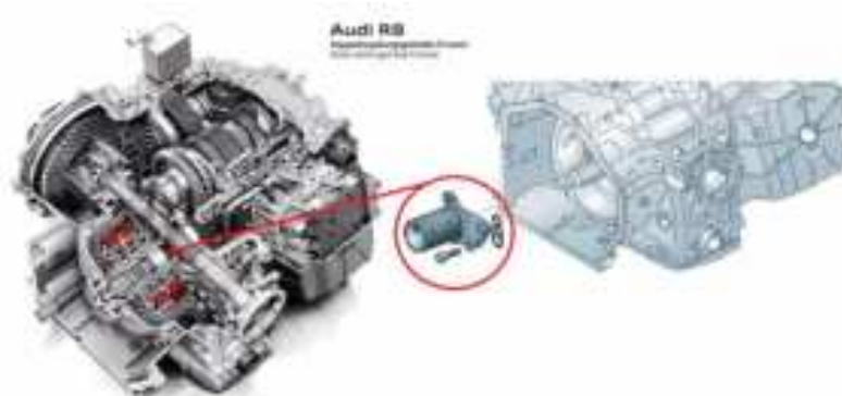
Fig. 1. The clutch carrier assembly (Kolenič et al., 2011)
