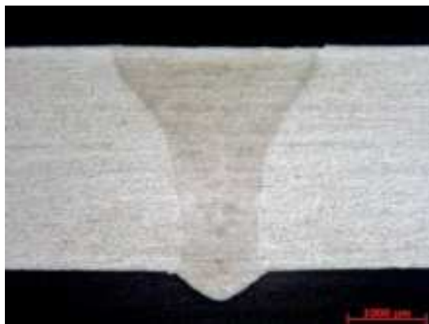
Fig. 11 Macrostructure of a welded joint produced by constant welding current
