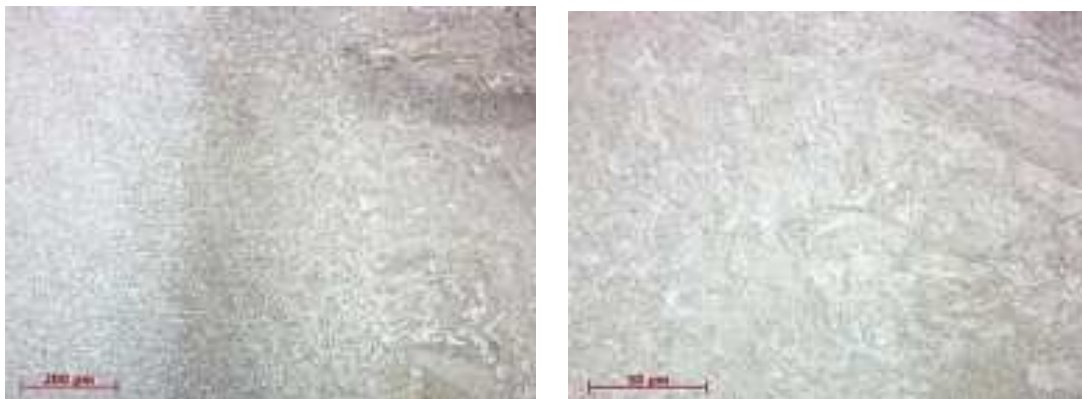
Fig. 12. Heat-affected zone (left) and fusion boundary in HAZ (right) on the side of base material S500MC
