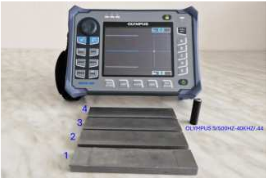
Fig. 2. NORTEC 600 device, OLYMPUS probe and experimental specimens
