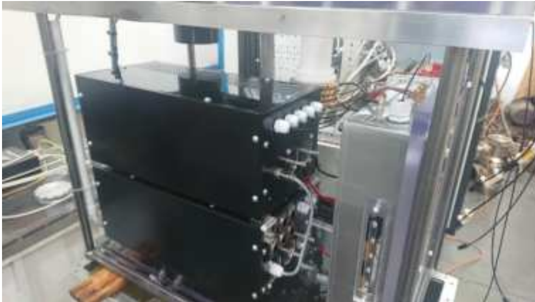
Fig. 5 View of a small container with active circuits at a high potential of 60kV
