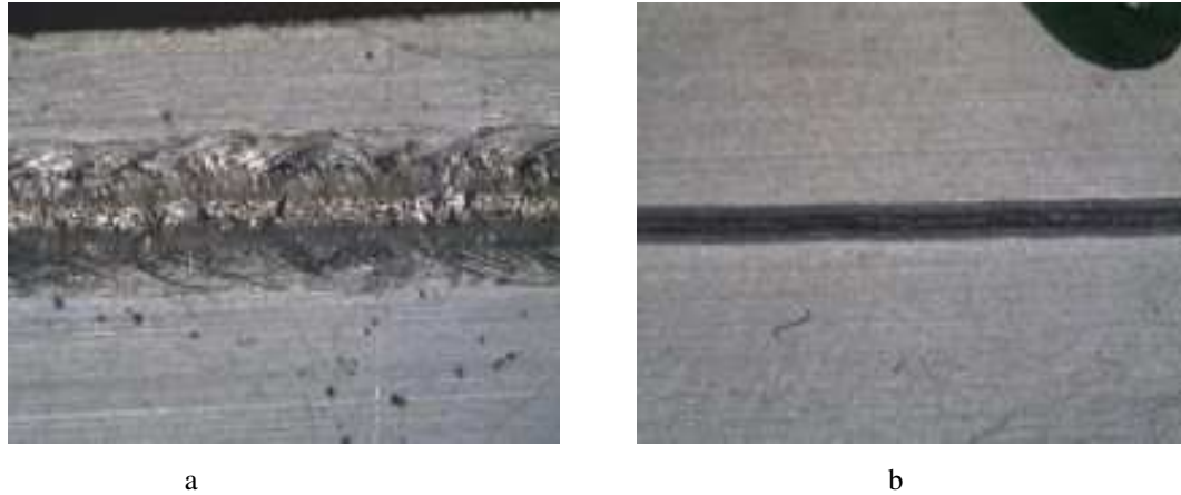
Fig. 6 Weld beads for parameters with v_z = 38.33 mm/s and P = 1500 W, with BL core:ring ratio: a – 100:0, b – 20:80
