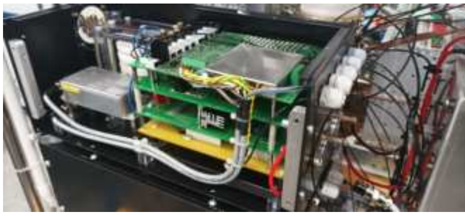
Fig. 4 Solution of the Wehnelt source at a potential of 60kV
