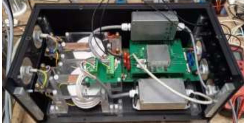
Fig. 13. The secondary part of the source is placed in a black aluminum box
