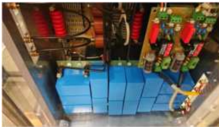
Fig. 1 Original concept – control node solution with passive components
