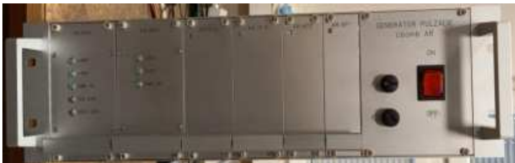
Fig. 12. The primary part of the pulse source with individual modules of the main and auxiliary source drivers
