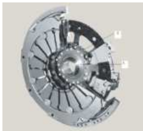
Fig. 2. Part of a car transmission 1 - steel hub, 2 – disc ( https://www.zf.com/products/en/cv/products_65885.html ).
